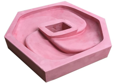
Silicone Mould— a soft elastomer silicone was chosen for relief of undercuts
