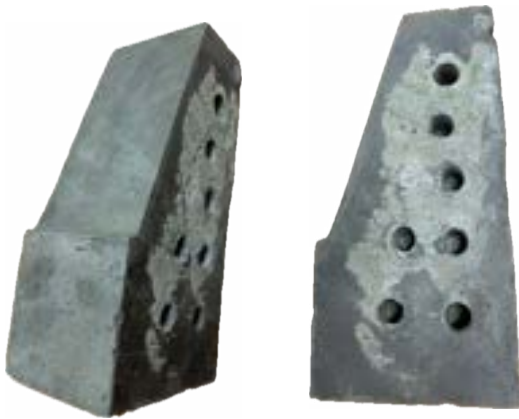
Original engineering brick pieces from client to match up for the architect
